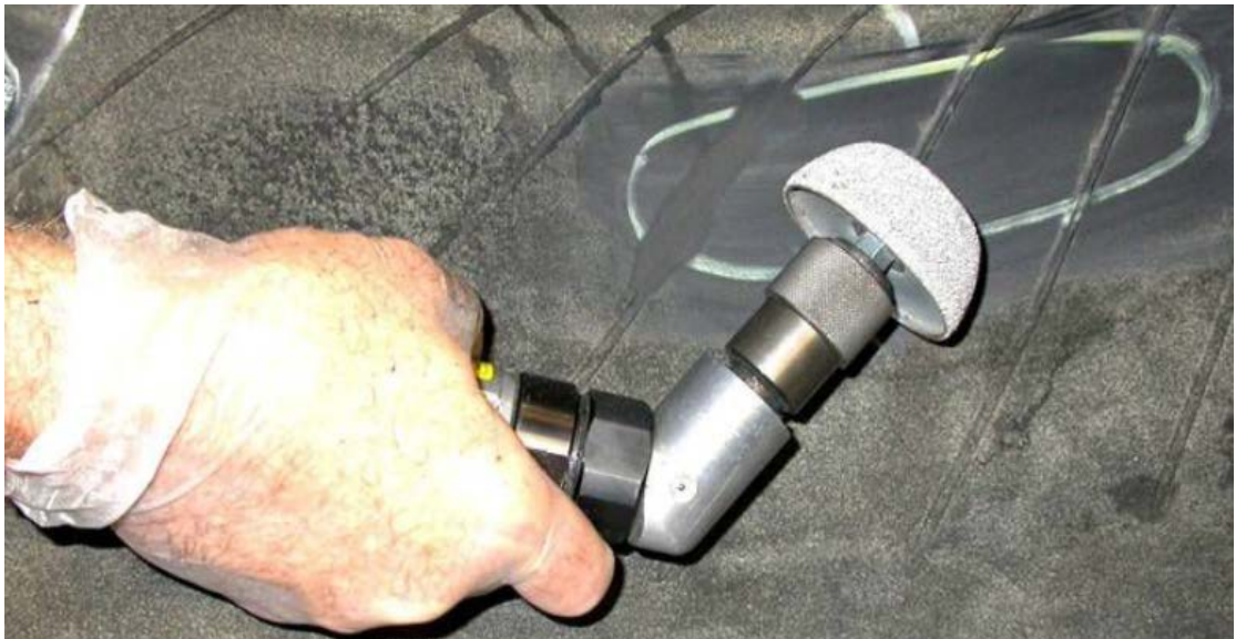
Buffing outlined area to achieve a smooth with Grinding Wheel
