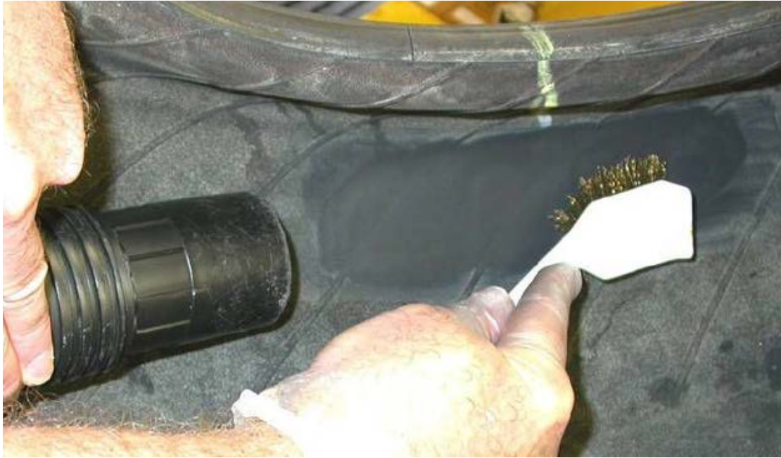
Using a brass-bristle brush and cleaner to remove buffing dust from the buffed area.
